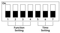
Note: The solid black blocks in the DIP switch diagrams indicate the switch positions. For example, all the switches are "off" in the diagram above.
